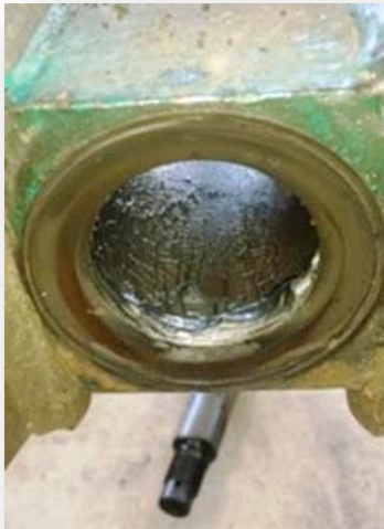
Figure 9: Wear in bore evidenced by grease pooling. Face wear into bore from washer movement.
