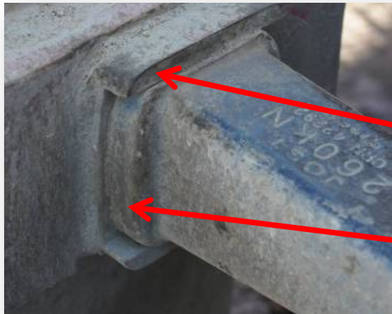
Figure 7: A drawbar eye with no visible wear or movement. Undisturbed paint around the drawbar eye indicates that there is no movement of the eye in the mounting block.
