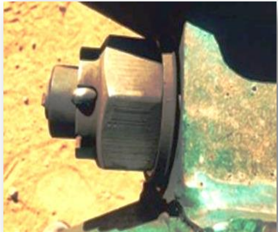
Figure 10: Mushrooming of the washer due to face wear into the bore.
