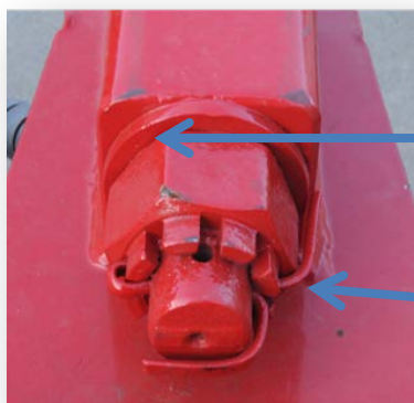
Figure 8: Correct bolt-in drawbar eye installation
