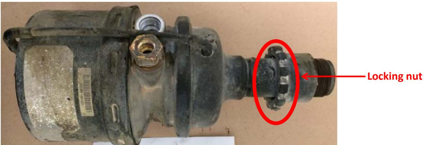
**Figure 1 – Affected brake actuator**
