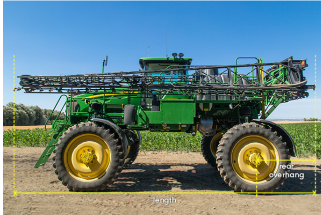
Figure 6: Example of an agricultural vehicles length and rear overhang
