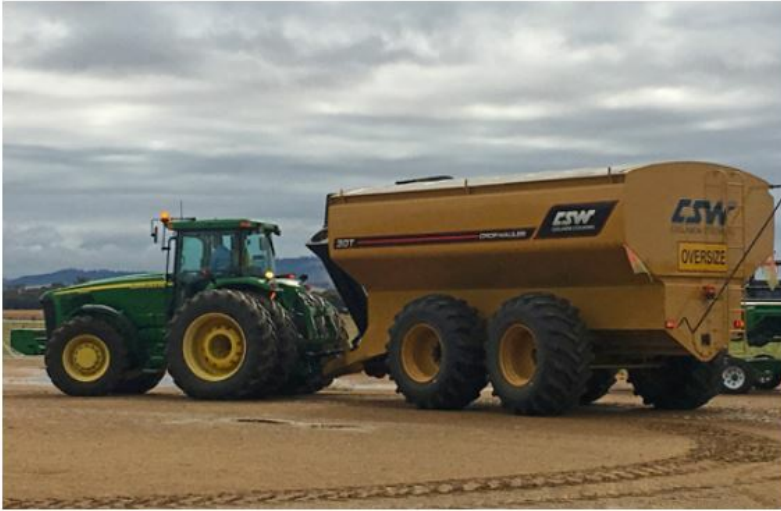
Figure 12: Example of the fitment of warning sign and a warning light fitted to the highest practicable point.
