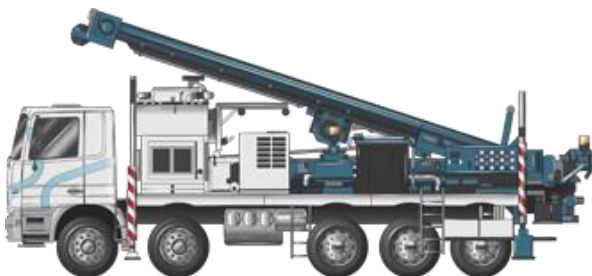
Figure 6: Truck Mounted Drill Rig 5 axle
