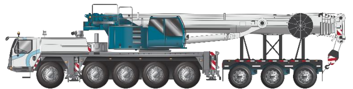
Figure 2: All Terrain Mobile Crane 5 axle and Boom Support Dolly 3 axle
