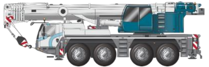
Figure 1: All Terrain Mobile Crane 4 axle
