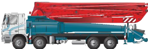
Figure 5: Truck Mounted Concrete Pump 4 axle
