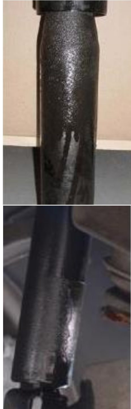
Figure 4.5 Examples of leaking shock absorbers
