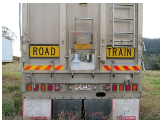
Figure 1: Road train trailers do not require a coupling fitted to the rear of the unit.
