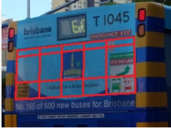
Figure 3: Breakable rear exit Red lines indicate where film should be cut or a gap left
