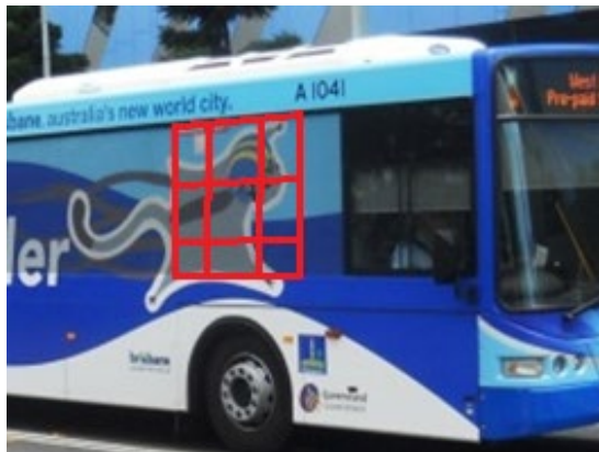
Figure 4: Breakable side exit Red lines indicate where film should be cut or a gap left (Courtesy of Dave Brown via Flickr)
